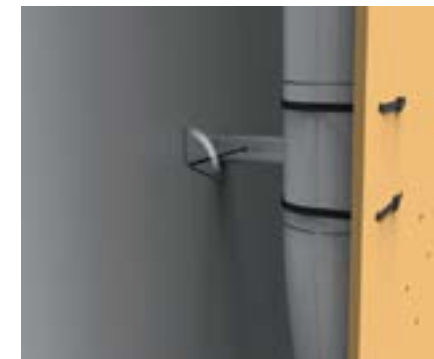
7. Detail of the wall pins fixing.
