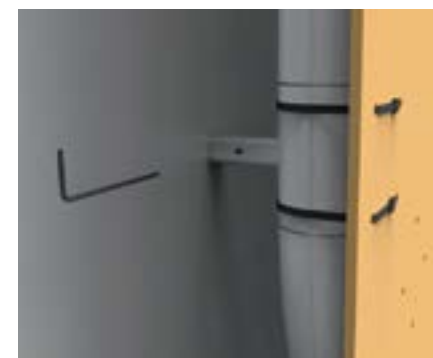
6. Detail of the wall pins fixing.
